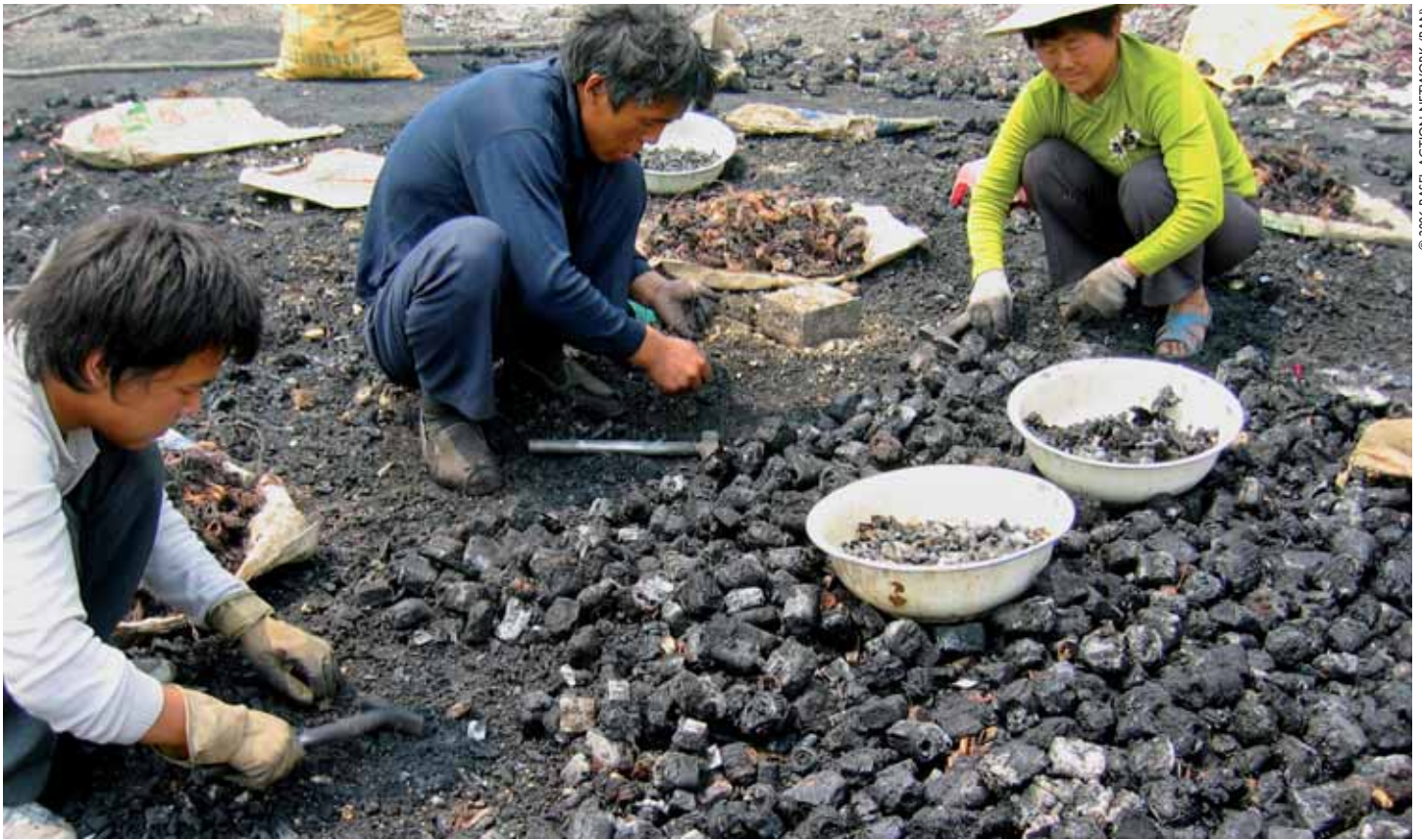
Workers crack piles of burned computer components to remove the copper inside unaware of the danger to their health.
